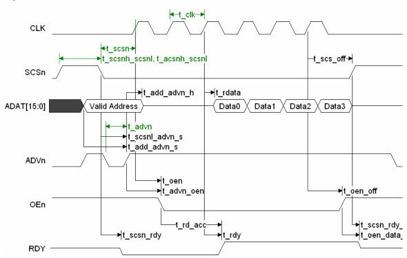
Notes: RDY going low is asynchronous to t\_scsn\_rdy. Going high, it is synchronous to CLK. Read Data output and RDY going high are synchronous to CLK. Valid Data Time programmable through Device Wait Count Register. Wait Count is not used for non-DMA synchronous reads.
